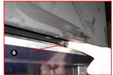
Figure 1: blocked stop lever
